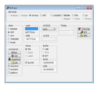
3. Enable Intel® PT on the target and allow TRACE32 to configure it.
