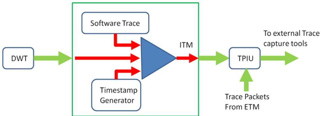
Each trace source is given a unique 7-bit Trace ID (ATID) so that the streams can be separated by the debug tools.
