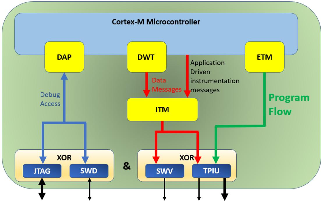
This is the block diagram for Cortex-M0+ devices.
