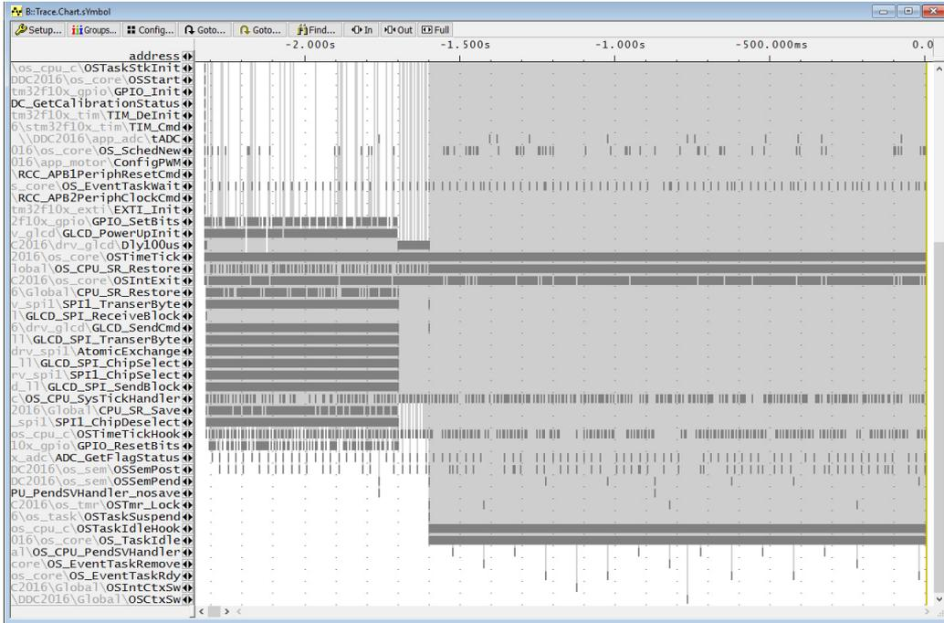
One of the features of the DWT is to be able to inject data trace events into the ITM for inclusion into the trace stream. The data events are configured using the TRACE32 breakpoint interface. More information can be found here: [“On-chip Breakpoints”](#), page 84.
