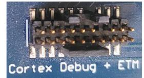
It is imperative to ensure that your development board has the correct connector for the debug features you wish to use. Other connectors are possible.
