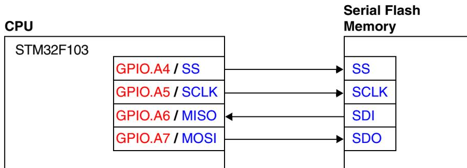
Using the commands below, the pins of the serial Flash interface (SPI) can be configured for the CPU STM32F103. The resulting configuration allows the CPU to switch from the GPIO A4-A7 to SS, SCLK, MISO, and MOSI.
