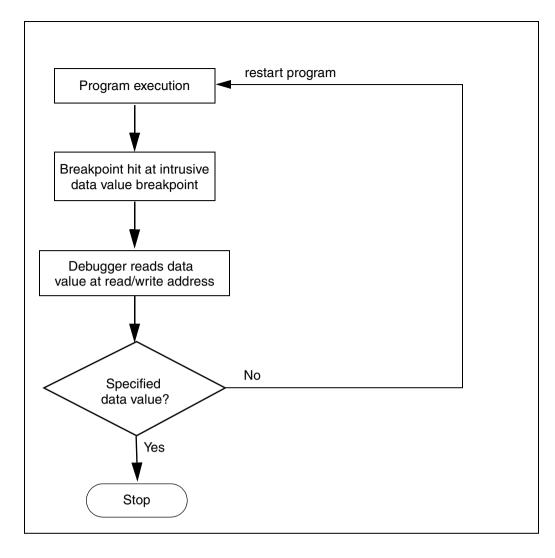
An intrusive data value breakpoint for "**break before make**" processors is implemented as follows:
