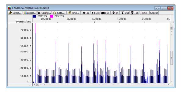
Example 2: In this script, an event counter recording is combined with an instruction flow trace recording.
