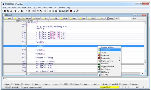
The TRACE32 GDB Front-End supports debugging the Linux kernel using KGDB. Please note that it is only possible to debug the kernel space. Debugging the user-space as supported by the TRACE32 Stop Mode Debugging for Linux is not possible.
