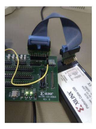
For information on setting up the Xilinx tools for using the TRACE32 debug interface for JTAG access, please refer to the application note "Using TRACE32 as backend for Xilinx tools".
