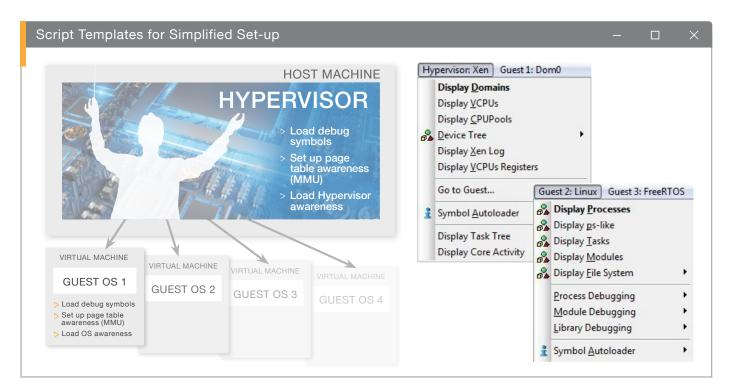
Lauterbach provides ready-to-use script templates to simplify the set-up process. After the communication between the TRACE32<sup>®</sup> debugger and the cores of the target system is established the following steps are required to configure hypervisor-aware debugging:
