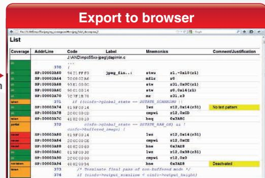
To collect data for code coverage analysis, the trace tool records all information about the instructions executed during the system test (**Record**). The recorded trace information is managed by TRACE32 PowerView in a code coverage database. This provides numerous ways in which the user can analyze and display the code coverage results (**Review**).
