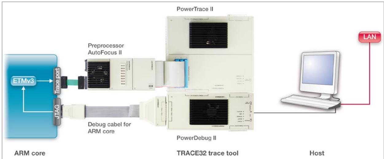
Fig. 6: The Lauterbach trace tool for long-term tracing with the ETMv3
