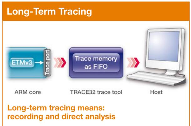
Long-term tracing is implemented by transferring the trace packages to the host during recording and analyzing them immediately. In this case, the trace memory of the TRACE32 trace tool is basically used as just a FIFO.
