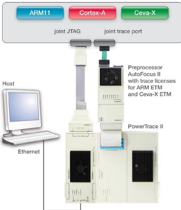
Fig. 16: A TRACE32 development environment for CoreSight Debug and CoreSight Trace
