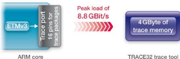
Fig. 3: The trace tool for the parallel ETMv3 supports a data rate of 8.8 GBit/s with 16 pins for the trace packages
