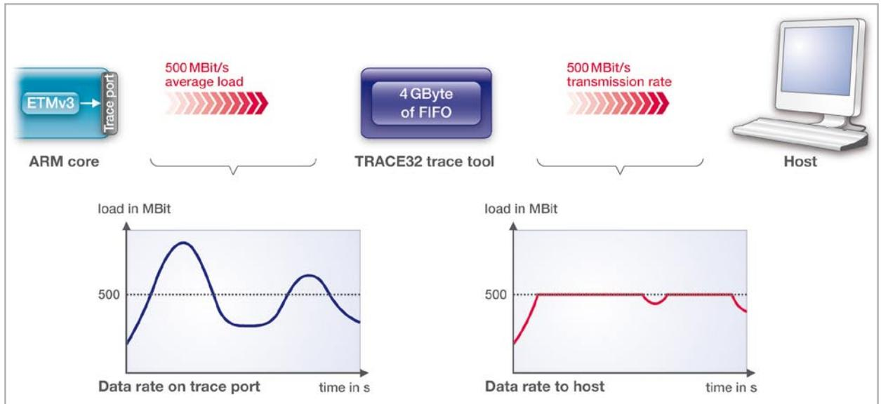
Fig. 5: Long-term tracing works for this example if the average load at the trace port does not exceed 500 MBit/s
