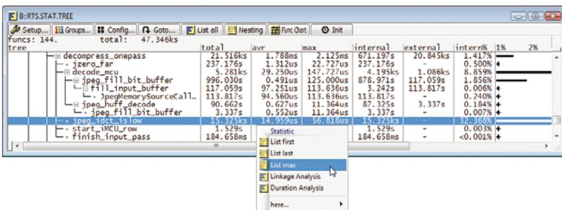
Fig. 10: If necessary, details on the longest function run can quickly be displayed
