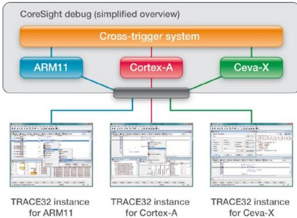
Fig. 14: A separate TRACE32 instance is started to debug each core
