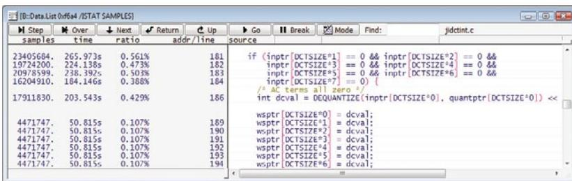
Fig. 9: Details of time behavior of program lines of a function
