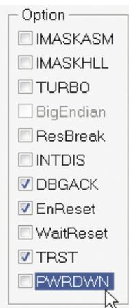
Fig. 9: The PWRDWN option, defining whether energy-saving modes are ignored or not during debugging
