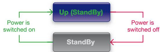
Fig. 10: Instead of issuing an error message, the debugger waits for power-up following a powerdown.
