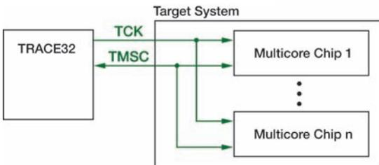
Fig. 7: The cJTAG interface, here for multichip target hardware
