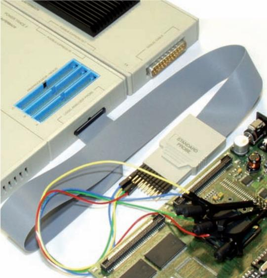
Since July 2006, PowerTrace II can be used not only to record the program and data flow but also to record up to 17 digital data channels or 4 voltage/3 current channels.
