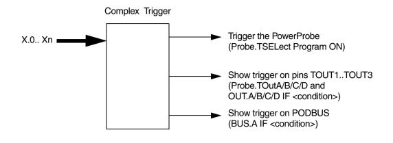
Like the PowerTrace, the PowerProbe also has a Complex Trigger Unit (CTU). To use the CTU you have to activate it by selecting the **Program** Checkbox in the advanced **Probe** window:
