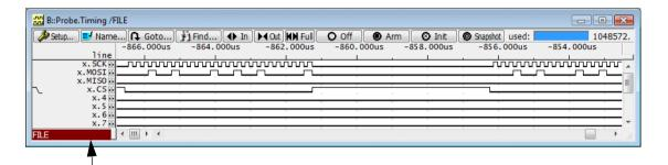
FILE in red indicates that the displayed trace contents was loaded with the Probe.FILE command
