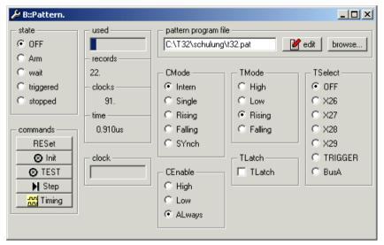
The Pattern generator has to be programmed via a pattern program file. Here is an example of such a file:
