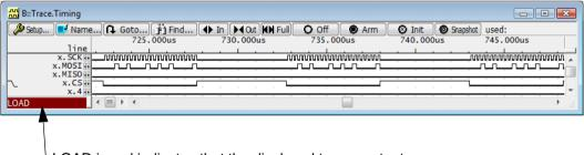
LOAD in red indicates that the displayed trace contents was loaded with the Trace.LOAD command
