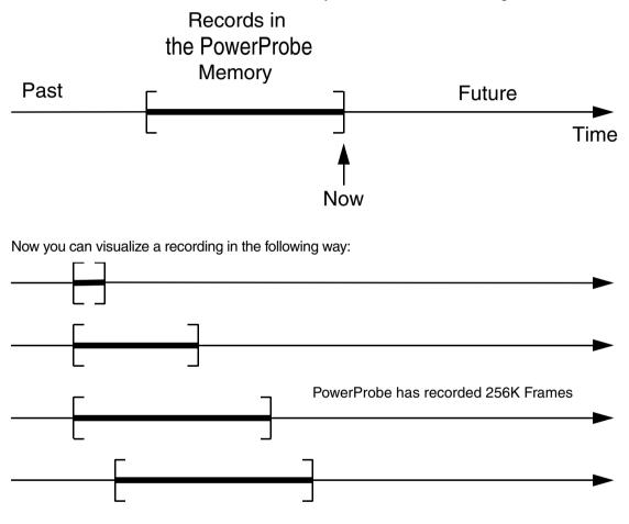
So at first the trace memory starts to fill up and after the trace memory is full, the window starts to slide.
