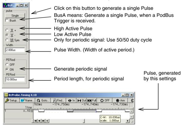
The output pin of the Pulse Generator is on the middle column of the PowerProbe and is labelled TOUT5.
