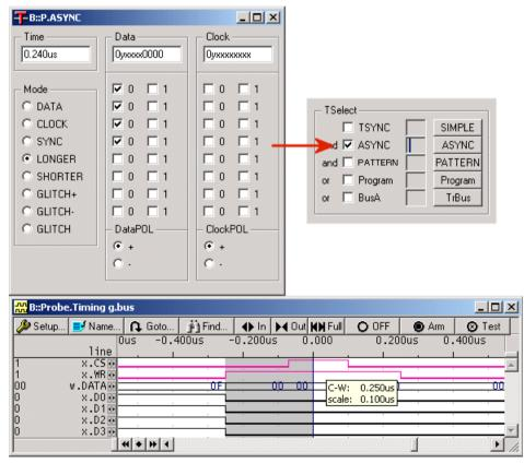
The input pins for this trigger are **x.0-x.7**. Internally the Async Trigger Unit generates two signals, which are called *DATA* and *CLOCK*. These signals are active, when the specified pattern is recognized on the input pins. For both signals it can be specified if they are active high or active low; this is selected with the **DataPOL** and **ClockPOL** settings. So the schematic of the Async Trigger Unit looks like this:
