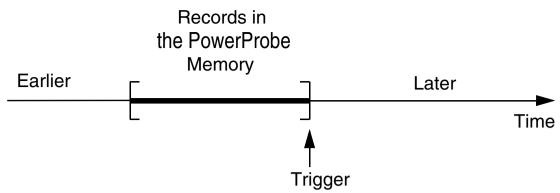
In this case you can see what happened before the trigger, but you can't see what happened after the trigger. To make this possible, you tell the PowerProbe to delay the break of the recording after a trigger has been detected. This TriggerDelay (**TDelay**) can be set in the advanced part of the **Probe** window:
