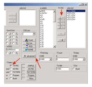
The checkbox TSYNC in the lower left corner selects the so-called Simple Trigger as trigger source.
