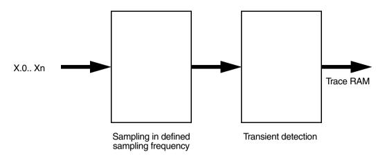
With the settings in the **Mode** box, you can change the sampling frequency of the PowerProbe. The default is **100 MHz** (100 MSamples/s). In this default mode all input pins are freely usable. When you select **200 MHz**, only input pins x.0-x.31 can be used. In **400 MHz** mode only input pins x.0-x.15 are available. In **50 MHz** mode, the PowerProbe lowers its sampling rate to 50 MSamples/s.
