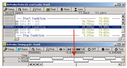
The **/Track** option also works to time correlate the trace data of the PowerProbe to the trace data of the PowerTrace. So with the **/Track** option you can correlate your program flow and data trace to the recording of your physical signals. There is some problem with this tracking: program flow and data traces are usually not very accurate and there usually is quite a big offset between the execution of an instruction and the generation of some corresponding trace data.
