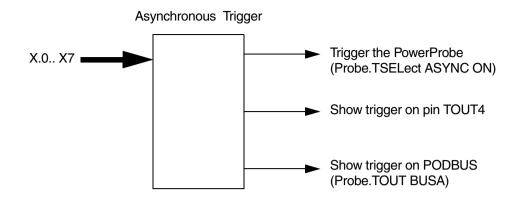
Additional to the Simple Trigger, there is also a so-called Asynchronous Trigger. It can be configured by clicking on the **ASYNC** button in the advanced part of the **Probe** window:
