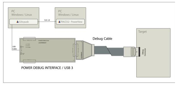
In order to implement this communication, the command line tool **t32tcpusb** has to be started on the PC to which the POWER DEBUG INTERFACE USB is connected. **t32tcpusb** can be found in the bin/<target\_os> directory of your TRACE32 installation (e.g. bin/windows64).
