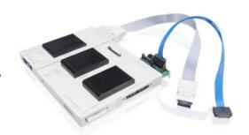
Or with *Preprocessor RH850 HSTP HF-Flex* and a PowerTrace II / PowerTrace III module. This configuration supports up to 4 lanes at a lower speed.
