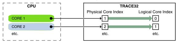
• Processors with physical e6500 cores and physical threads, e.g. T2080:
