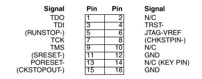
This is a standard 16 pin double row (two rows of eight pins) connector (pin-to-pin spacing: 0.100 in.). (Signals in brackets are not necessary for basic debugging, but it is recommended to take them into consideration for future designs.)
