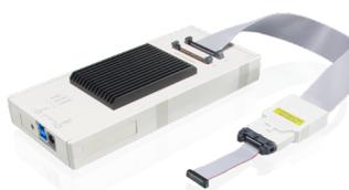
**2** All-in-one Debug- and Trace-Tool for Cortex®-M
