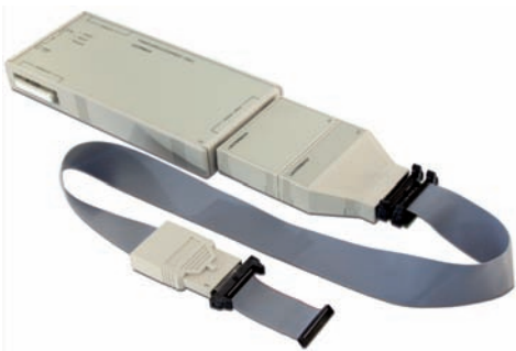
Fig. 9: PowerDebug Module and CombiProbe as low-priced development tools for the Cortex-M series
