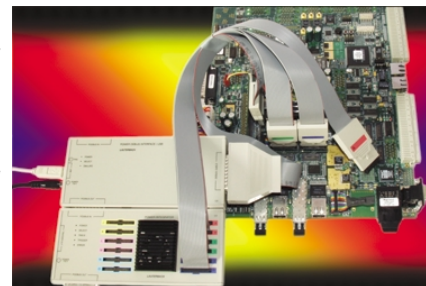
Figure 4: TRACE32-ICD in-circuit debugger and PowerIntegrator on a PowerQUICC III evaluation board
