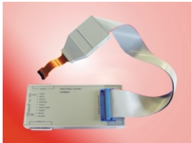
Preprocessor in casing with Flex-Extension for easier connection to the target system
