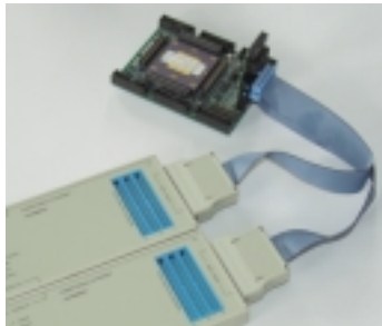
Figure 1: Two independent Lauterbach debuggers that debug an SoC with two cores via a joint JTAG interface
